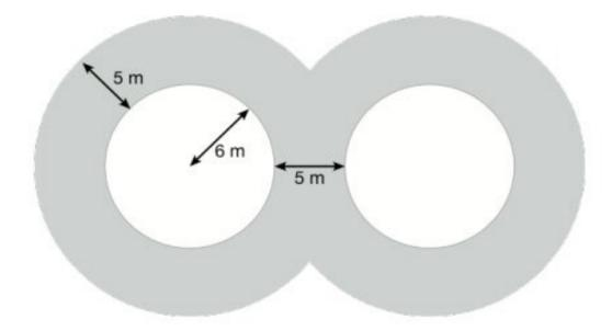
2.20.2 Solar cars must be able to negotiate a slalom course in less than 11.5 seconds.
